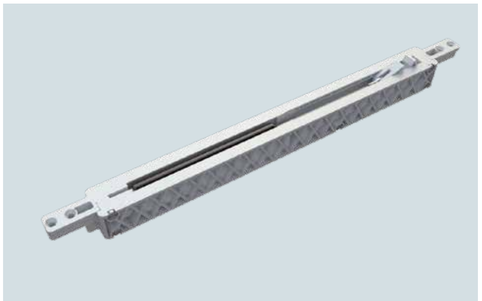
SOFT CLOSE DAMPER: THIS BRAKES THE SASH GENTLY JUST BEFORE THE END POSITION AND THEN PULLS IT SHUT AUTOMATICALLY.
